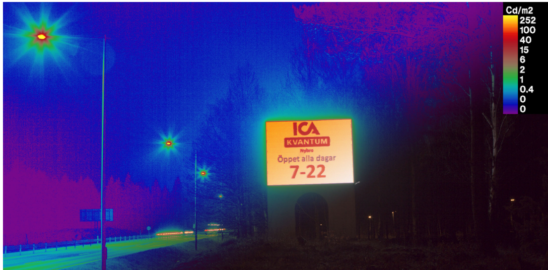
Figure 4: Measuring the average surface luminance of an advertisement sign to comply with CIE 150:2003 or EN-12464-2
