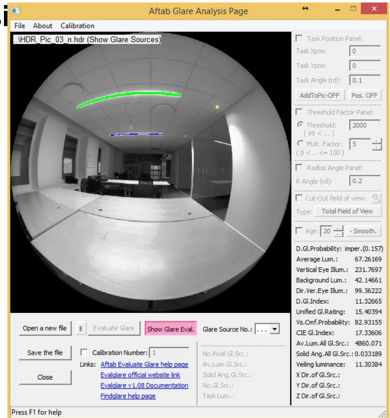
Measuring UGR by using the Evalglare interface page in Aftab-Alpha software.
