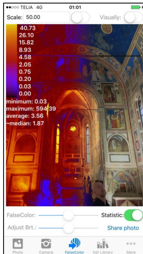
Figure 3: FalseColor page in Aftab Luminance iPhone app. It shows the falsecolor images with different pallets. It also gives us the minimum, maximum, average and median luminance value of the whole image.
