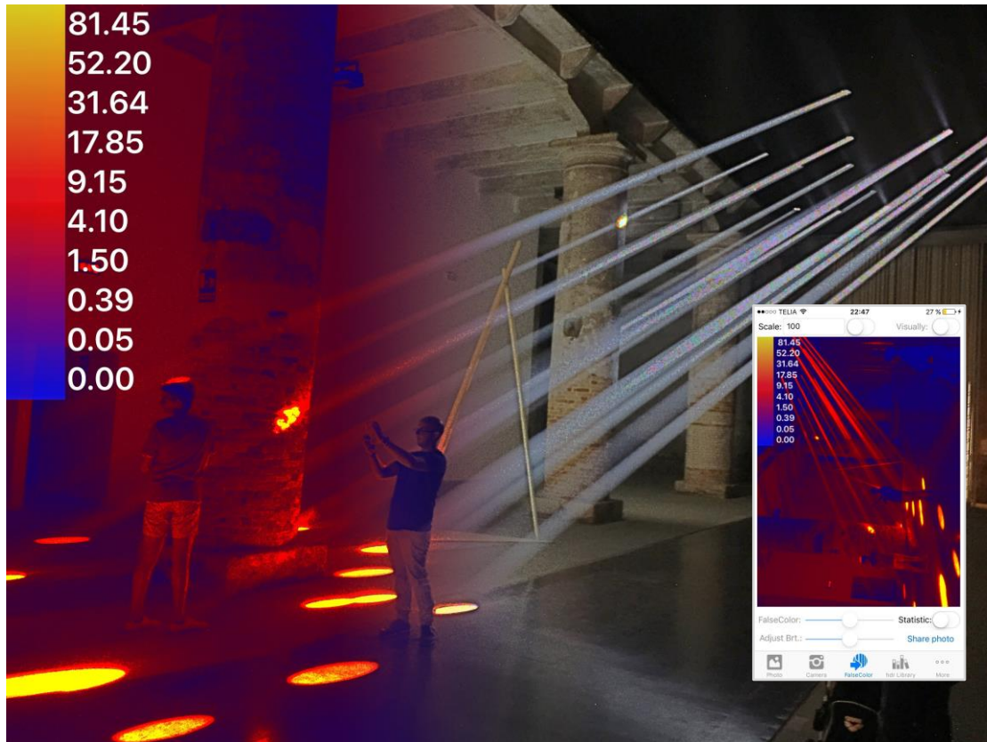
Figure 1: A photo that is taken by Aftab Luminance iPhone app in Venice Architecture Biennale 2016. Such a photo realistic HDR image can help us to get the luminous information of any environment immediately.
